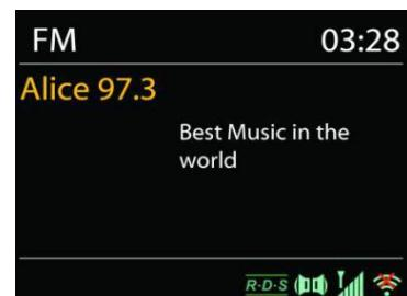
FM radio mode receives analogue radio from the FM band and displays RDS (Radio Data System) information about the station and where broadcast.
